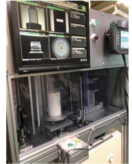
Appearance inspection using a high-sensitivity camera
